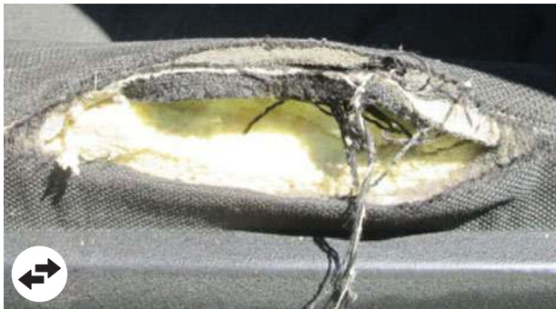
Foam missing or broken frame
