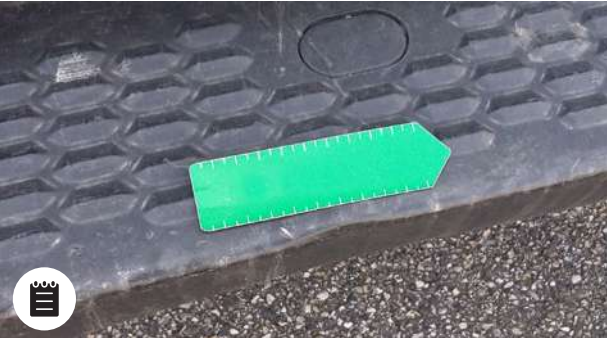
Rear Step Slight deformation
