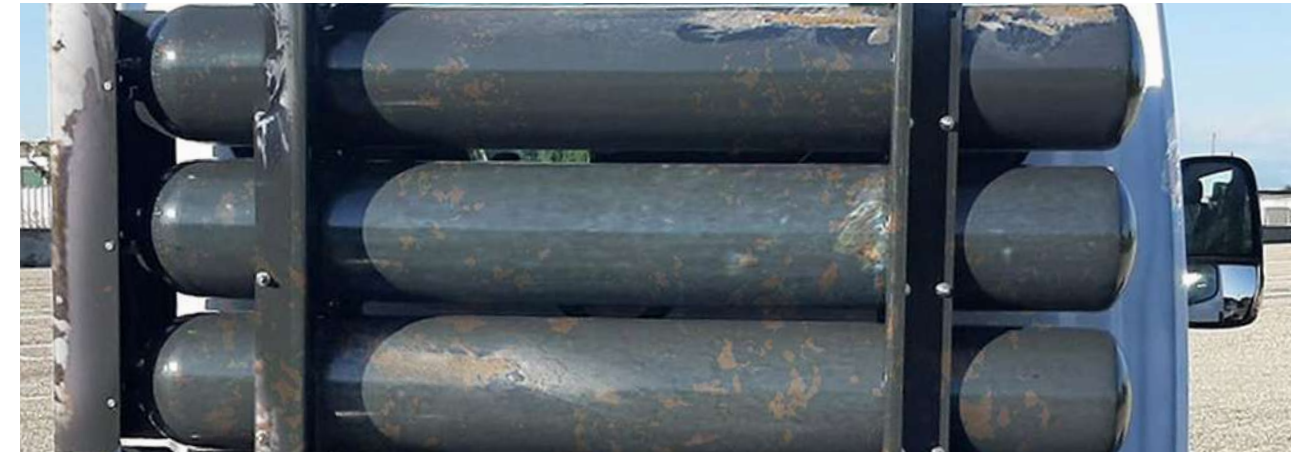
Evidence of repairs to the CNG cylinder → charge for replacement for CNG cylinder.
