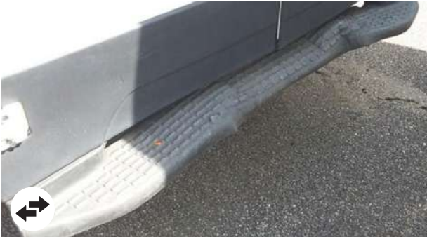
Rear footboards: Deformations not within economic repair
