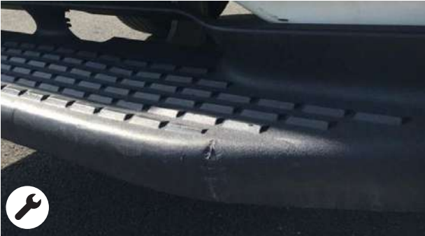
Rear footboards: Deformations within economic repair
