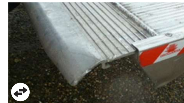
Tail lift: Deformations of platform within economic repair
