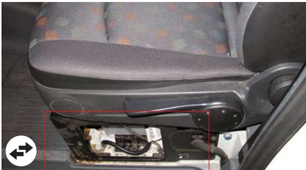
Missing equipment or trims
