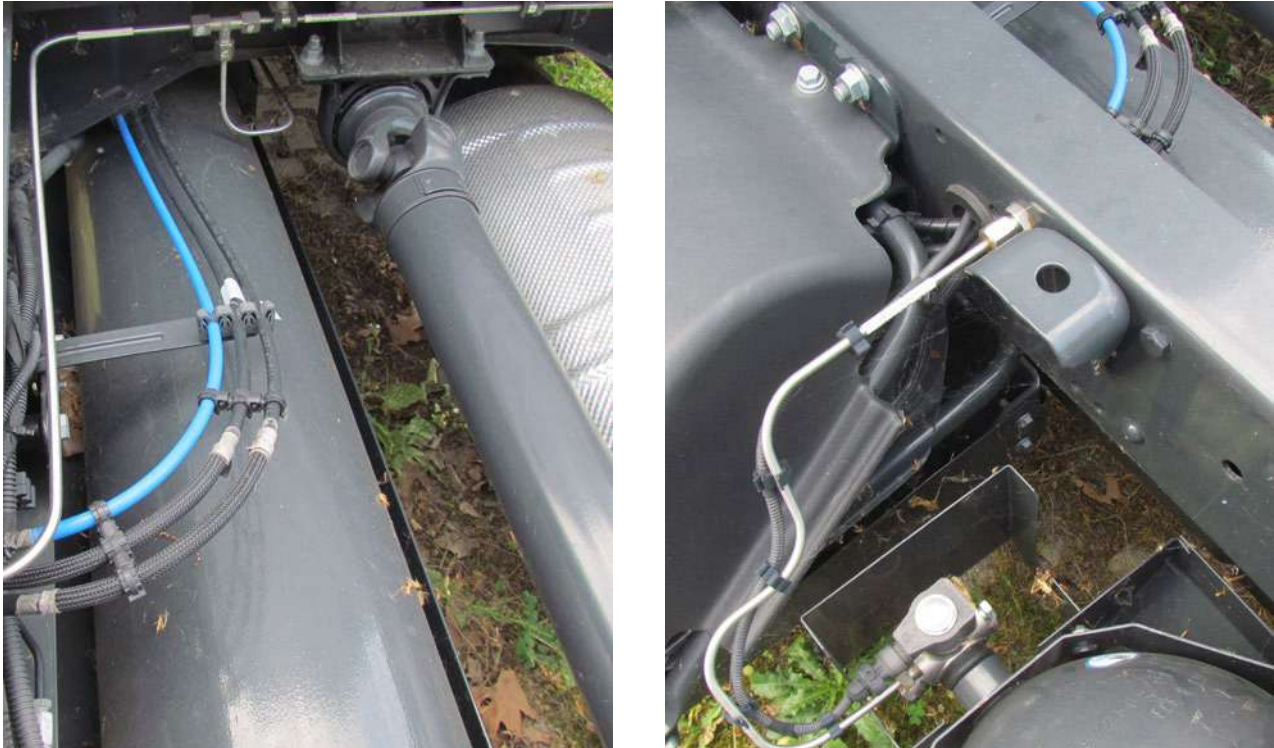
Check integrity of the gasoline fuel lines (no losses, no evidence of deep scratch). Fuel lines must be returned in proper conditions as illustrated in picture.
