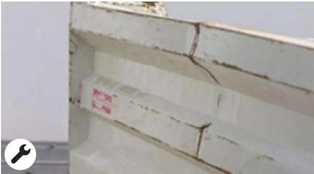
Deformations in the body closures with a repair time > 1 h within economic repair
