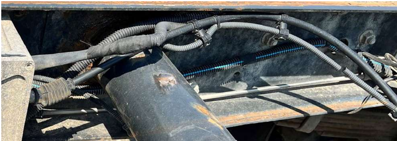
Losses or evidences of deep scratches charge for replacement of fuel lines.
