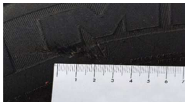
Tyres: Notch \leq 3 mm deep (CONFORMS)
