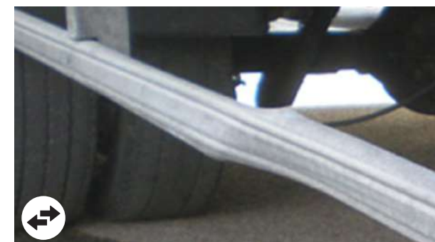
Side underun guards: Deformation beyond economic repair
