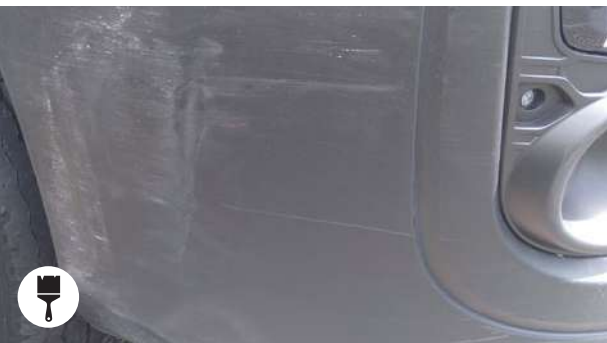
Scratches that can be felt with your nail and surface > 45 cm² (equivalent to a credit card)
