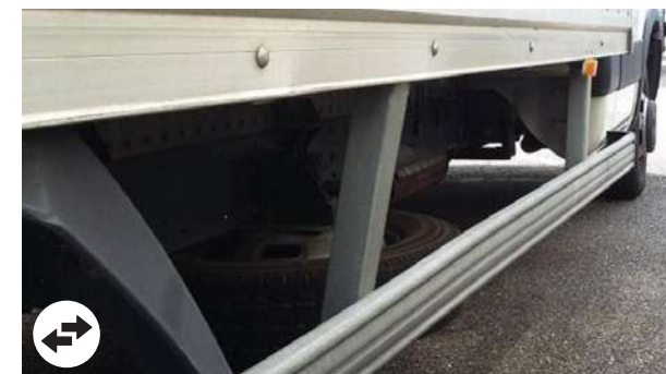
Side underun guards: Deformation within economic repair
