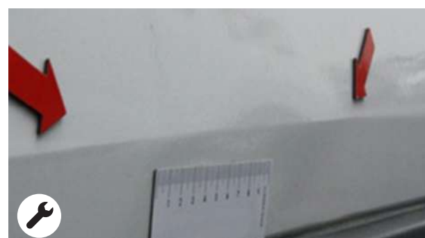
Defect: Deformed panel following repair
