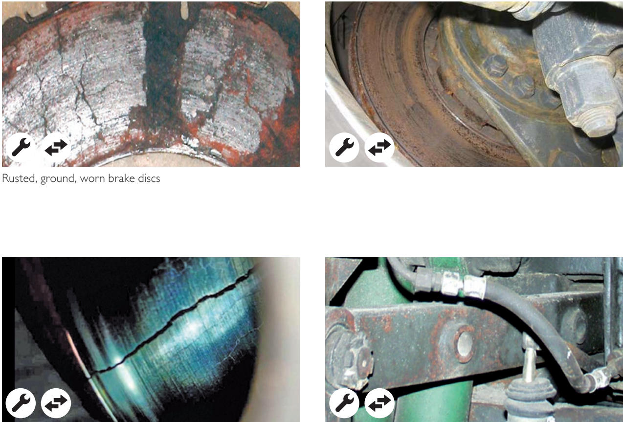
Does not conform to highway code and not valid during technical check
